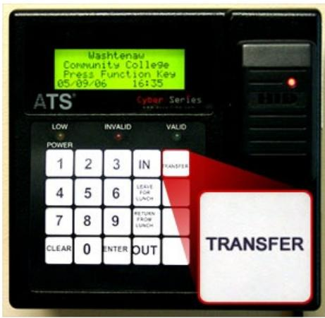
a. Press "TRANSFER" on keypad and the "Transfer" screen will appear.
