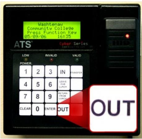
a. Press OUT on keypad and the "Clock OUT" screen will appear.
